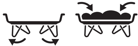
Animation showing when pan legs should be set in the unfolded position
